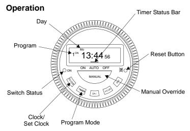
N.B. Before programming or setting the clock for the 1st time press the RESET button.
