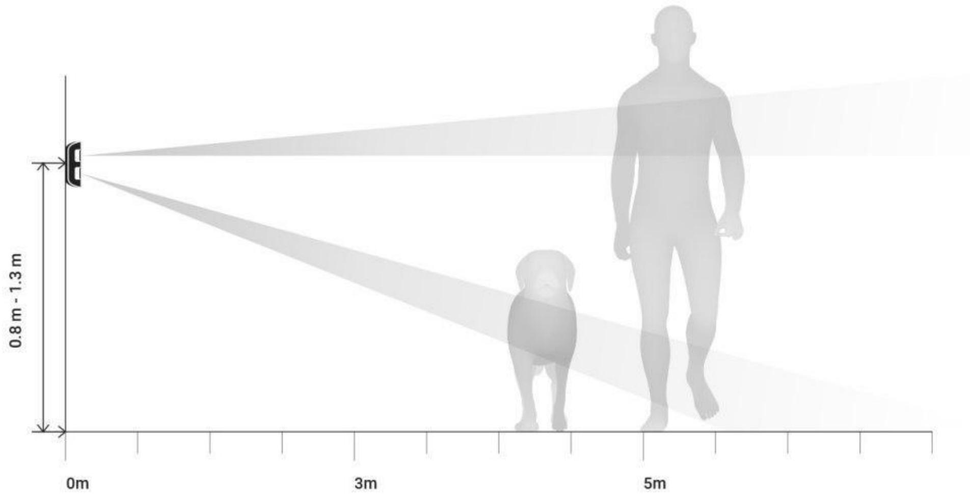
The detector recognizes motion and sends the first alarm immediately, but next alarms until disarming are transmitted no more than once in 5 seconds.
