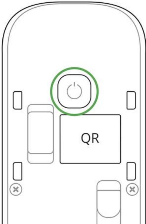
For the detection and interfacing to occur, the detector should be located within the coverage area of the wireless network of the hub (at a single protected object). Request for connection to the hub is transmitted for a short time at the time of switching on the device.
