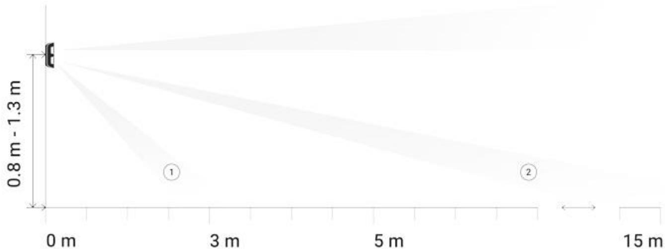
*The lower PIR sensor beam direction with the specified minimum (1) and maximum (2) detection range*
