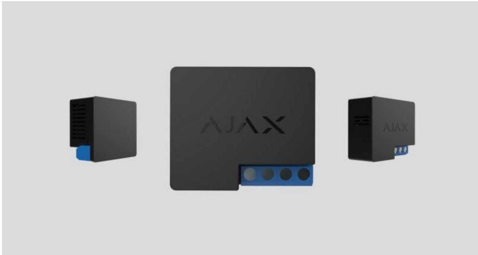
**WallSwitch** is a device that combines a wireless power on/off relay for electrical appliances and a power consumption meter. The miniature body of the device is adapted for installation in a European type socket.
