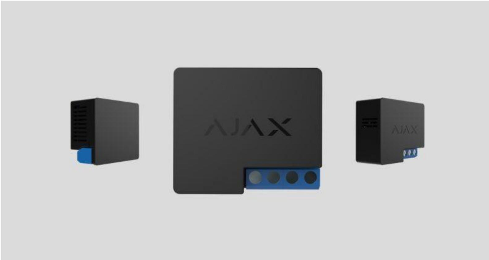
**Relay** is a wireless relay with a potential-free dry contact intended for switching appliances and devices on and off, powered by a 7–24 V DC source. The relay also has a pulse equipment control function. It is connected to the Ajax security system by the Jeweller secure protocol, the distance range is up to 1,000 meters if there are no obstacles.
