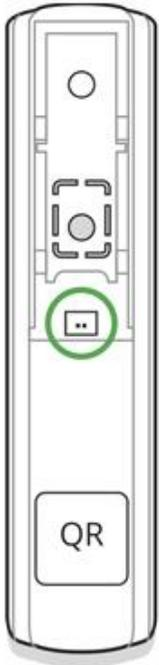
We recommend to install a wired detector at a distance not exceeding 1 meter – increasing the wire length will increase the risk of its damage and reduce the quality of communication between the detectors.
