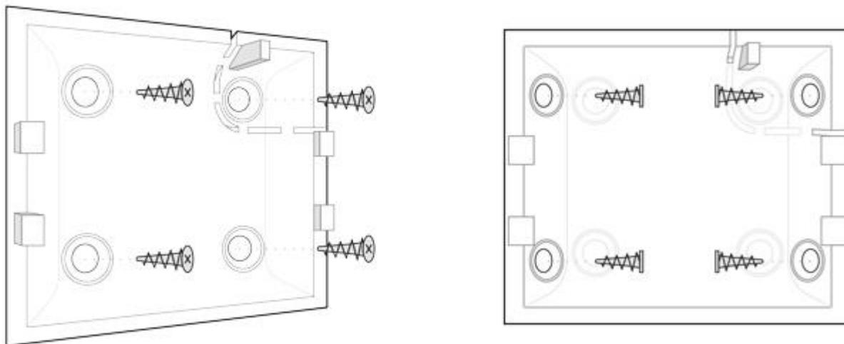
1. Attach the SmartBracket panel to the surface using bundled screws, using at least two fixing points (one of them – above the tamper). After selecting other attachment screws, make sure that they do not damage or deform the panel.
