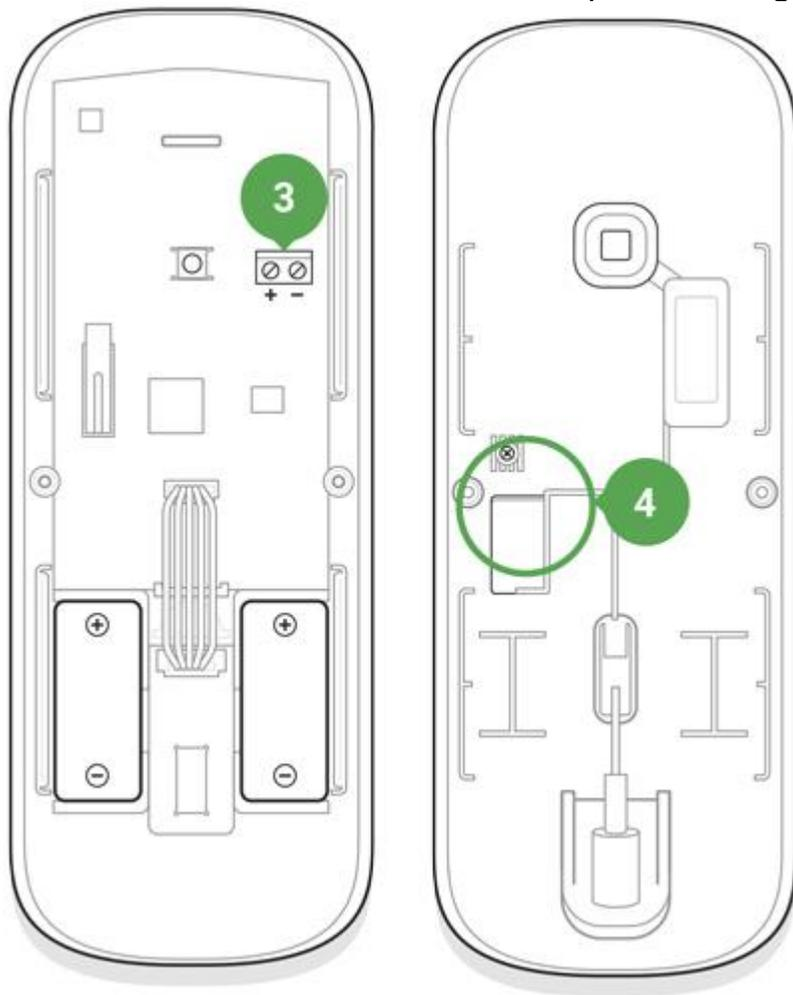
3. Terminal strips on the detector board
