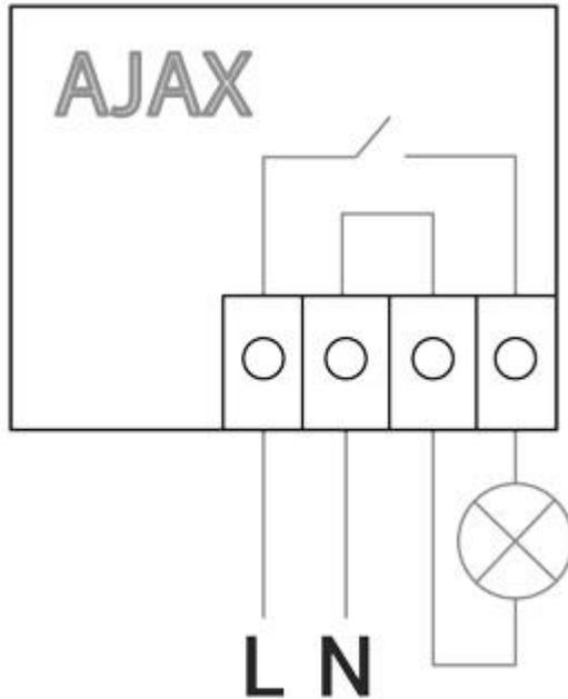
3. Connect a socket to the WallSwitch using bundled connecting wires or an electrical appliance using a cable with the sufficient cross-section. It's recommended to use cables with cross-section of 1.5 – 2 mm<sup>2</sup>.
