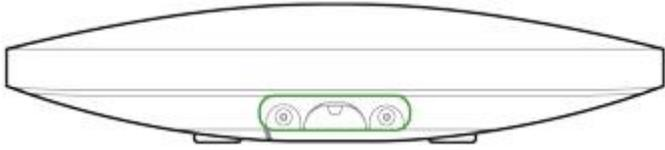
Fixing the hub on lid with screws prevents any accidental shifting of the hub and minimizes the risk of device theft.
